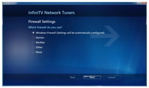
The Firewall settings are automatically configured for Windows Firewall. Selecting another option lists the required port settings for other Firewalls. These must be configured manually.
