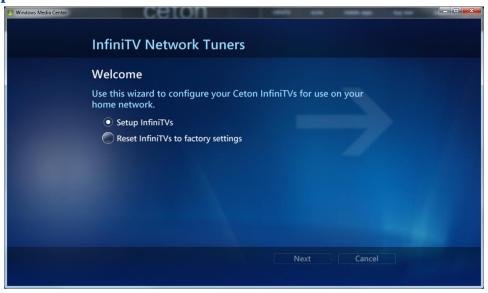
Select **Setup InfiniTVs** to proceed with Network Tuners setup. **Reset InfiniTVs to factory settings** will reset all InfiniTVs on the network back to their original settings and can be useful if you're having problems with your InfiniTV device.
