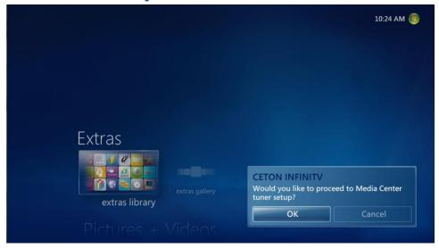
Media Center tuner setup must now be run in order to configure the selected tuners for use with this PC with Media Center. The Microsoft Digital Cable Advisor must be run on each PC which will be used.
