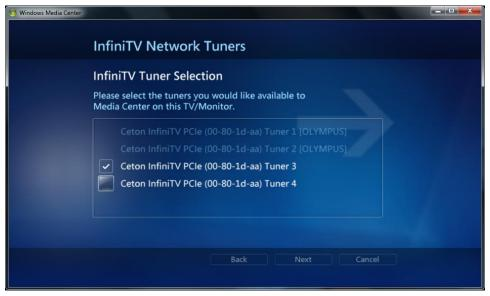
After setting up Network Tuners on the Host PC, the Network Tuners wizard must be run on each Client PC as well to configure those PCs for receiving cable TV. Follow Steps 1 to 9 above on each Client PC. Only tuners which have not been previously selected for use on other PCs will be available. Tuners previously selected are grayed out with the PC assigned to each tuner shown (see above).
