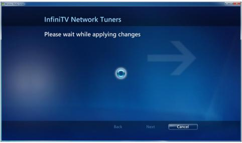
Applying changes sets up the network and assigns the selected tuners to this PC.
