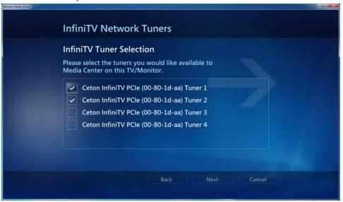
Select the tuners to be assigned to the TV/Monitor attached to this PC. In the above example, Tuner 1 and Tuner 2 have been selected for the Host PC, leaving Tuner 3 and Tuner 4 available to be used by one of two Client PCs elsewhere on the network.
