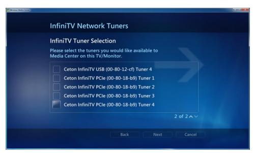
If you have multiple Ceton InfiniTV devices installed on the Host PC, the Network Tuner wizard will identify all of them and you can choose which tuners will be assigned to the Host PC and which tuners will be assigned to any client PC(s). You can even mix and match InfiniTVs with different interfaces (PCI Express and USB), as in the example above.
